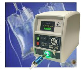
If the part passes the leak test, the Connects automatically release the part to the operator. If the test fails, the part is securely held in the Connects and requires a reset action of some kind (operator pressing the Stop button or requiring a key reset) to unlock the part. This action is used to prevent the inadvertent placement of the failed Bags into the passed-part area.
