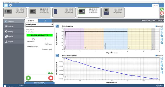
Screenshot displaying an instrument's last test cycle with plots of the captured data
