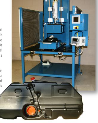
Any leak path from the inside of the tank to the chamber surrounding the tank would cause it to lose vacuum or gain pressure from the atmosphere. The chamber also serves to support the tank and minimize stretching, thus increasing testing sensitivity and reducing the potential for test error. The
