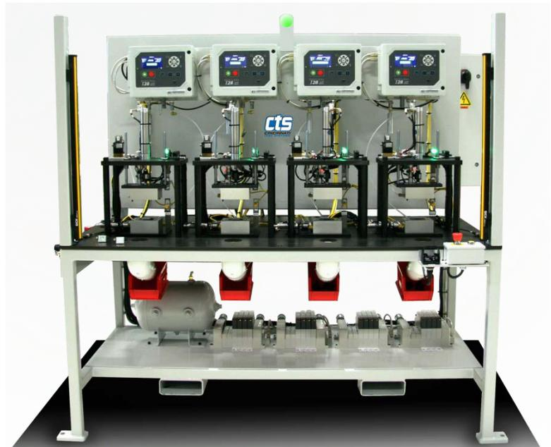
***Four-station volumetric fill pressure decay system testing electronic sensors to IP67 standards***
