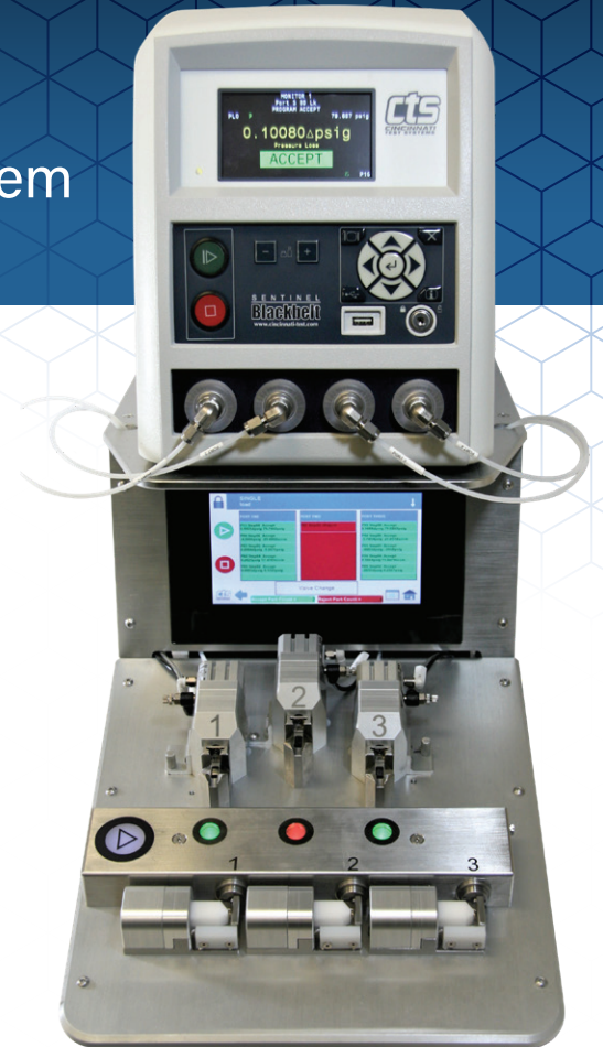
Benchtop testing system utilizing 4-Port Sequential Blackbelt for testing non-finished (untipped and no skived holes cut) multi-lumen CVC or PICC Catheters for both leak and blockage.
