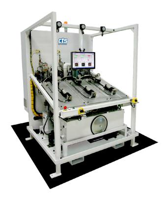
Functional testing is utilized to measure the performance of complex assemblies. A functional test system applies force and power to the part under test to measure its output compared to its tolerance to ensure that it performs within its specification.
