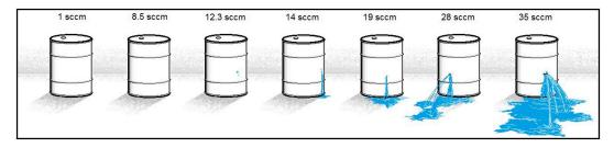
Then pressurize the parts with water (or the typically contained fluid) at the same working pressure and observe them for the agreed-upon cycle time established for a part that "doesn't leak." If the parts had a wide variation in air leak rates, they will exhibit different magnitudes of liquid leak.
