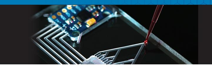
Microfluidic chips are used in a multitude of biological diagnostic applications, including analytical separation, detection, fluid control (sampling/mixing) and more. Once placed within durable analytical instrumentation, these devices typically have multiple unique micro pathways isolated from one another for liquid media passage, sampling and analysis.
