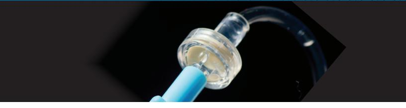
Check or one-way valves allow liquid flow in one direction and resist reflux, or back-flow, in the opposite direction based upon the presence of an internal elastomeric "duckbill" valve or an elastomeric disc. This elastomeric valve is often housed in an injection-molded polymer/plastic body which is either ultrasonically welded or adhesively bonded.
