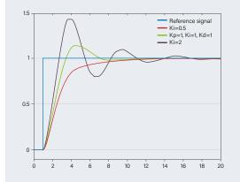
**Integral:** Affects the acceleration toward the target pressure. This uses the magnitude and duration of the error to determine acceleration.
