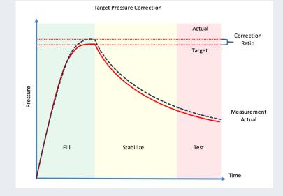
Target pressure correction paired with a robust calibration cycle allows for a precise and repeatable test measurement. The instrument achieves this by collecting all the data points measured during the test cycle. The calculation of loss uses a linear regression algorithm supplying precision measurements of small pressure changes over a long period of time. By combining target pressure correction into this algorithm, noise commonly measured over long test cycle times is removed.
