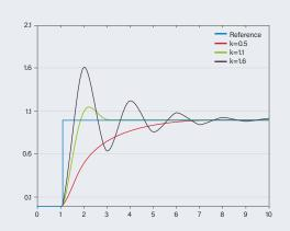
**Proportional:** Affecting the gain of the controller; the larger the error from the setpoint, the larger the proportional effect.
