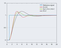
**Derivative:** Controls the setting time and stability of the system, which is not often used due to other methods of filtration like low pass filters.
