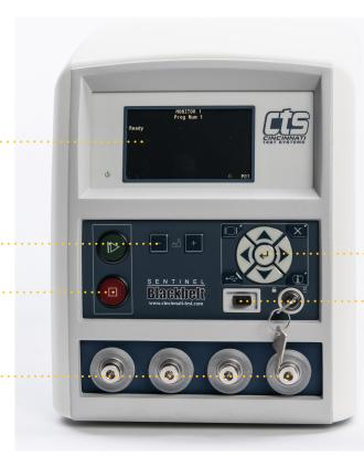
Monitor Selection Button, Exit Button, Enter and Navigation Buttons, USB Button, Information Detail Button
